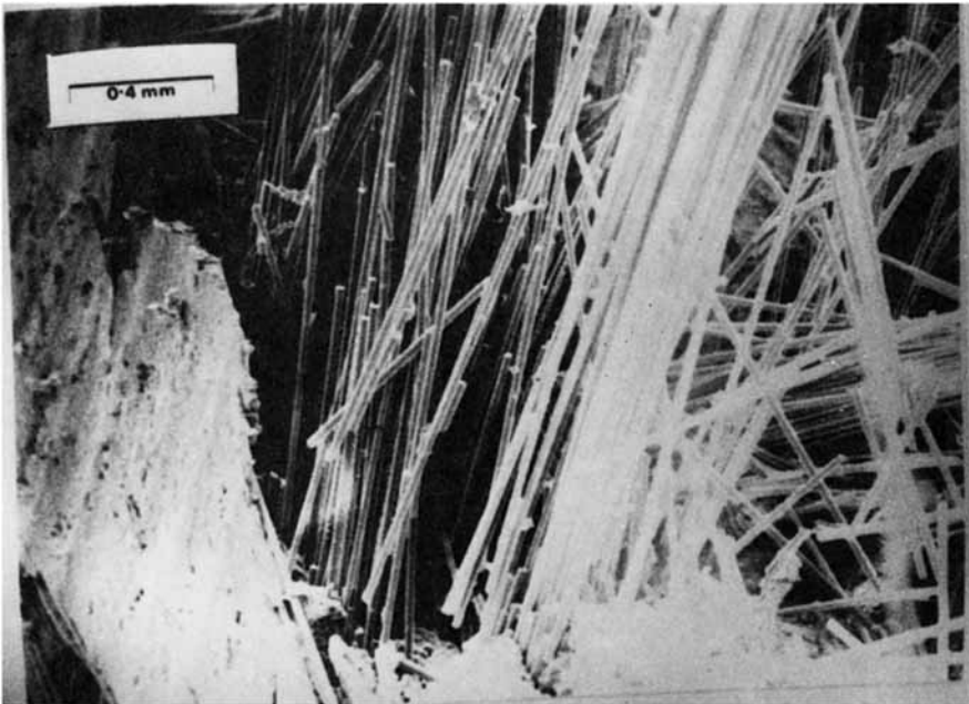
Fig. 12. SEM of impact fracture surface showing extent of fiber pullout.
